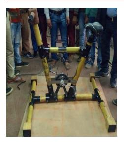
Tool Room & Training Center (TTCR), Patna has developed an innovative model of Gym Cycle using Bamboo. Design has been modified replacing some of the parts of Gym Cycle with Bamboo and provisions have been
