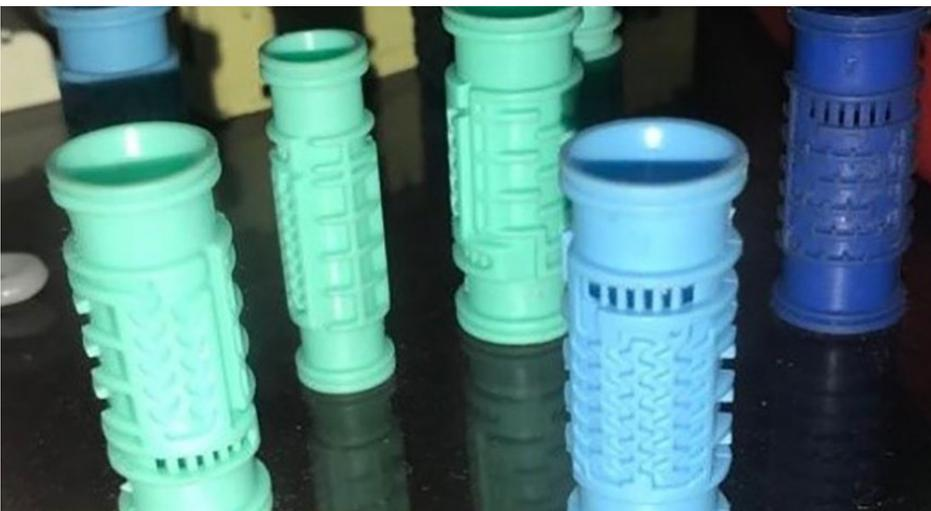
A Multi Cavity Mould has been designed, developed and manufactured for drip irrigation system. These components are being used for optimum drip watering for tea
