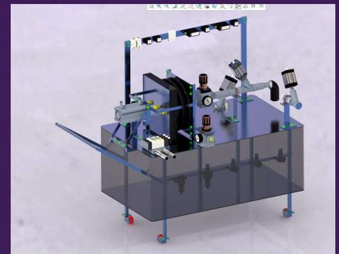
3-D Base Model of CPAP Type Ventilator
