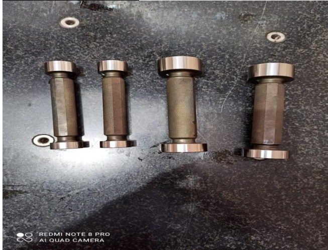
Product: Precision Plug Gauge for TA Link, Customer: M/s. Metal and Steel Factory, Ichapore
